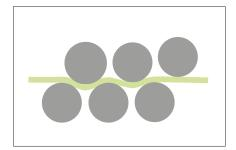
The COMPACT series has 6 manual straightening rollers to remove coil set and give customers flat material every time. The rollers are made of polished steel with a 70 mm diameter.
