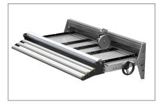
The infeed guide roller are angled to match the loop of the coil from a decoiler. This helps prevent creasing on soft materials like copper, aluminum and zinc. Another helpful feature is guiding the coil into the infeed guides. Between the slitter and shear are roller guides to ensure the material guides into the shear without curling up.
