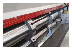
5 Sets of slitting knives come standard on the Compact series slitters. The unique "Cap-Locking" system gives you trouble free slitting the life of the machine.
