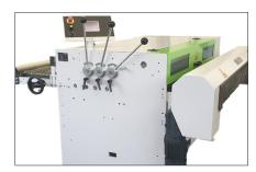
The coil guide is an important component for the function and accuracy of every system. The table has fixed and a manually adjustable coil guide with ball bearings. The adjustment of the movable coil guide is done by a hand wheel. This specific table has rollers integrated in the table to ensure a smooth surface.
