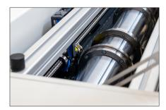
With the unique system for automatic setting of the position of the slitting knives and blade gap, you will get perfect strips in a minimum of time.
