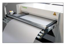
With the STRAIGHT extension, the material is fed smoothly, and the integrated straightening (optional) results in completely flat strips without stop marks. With straightened strips, you facilitate the feeding of your folder and secure the quality of your trims and panels.
