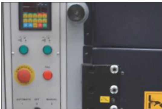
The MG line mechanical shears are standard with NC control which provides "multi-step" and "touch and go" programming features for the backgauge.
