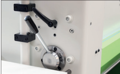
Simple and clear blade gap adjustment for varying thicknesses.
