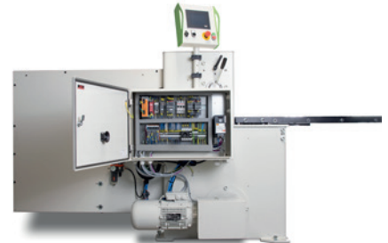
Service friendly with easy access to control, electrical cabinet, electronics and air.
