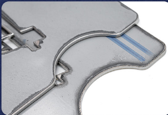
Edge rounding of foiled parts without damaging the protective foil
