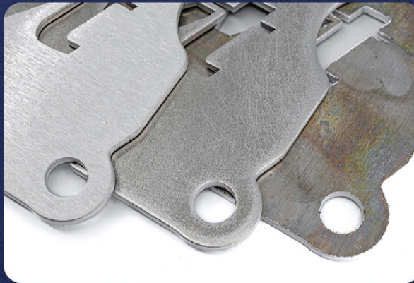
Deburring and edge rounding of the aluminium parts including final surface finishing
