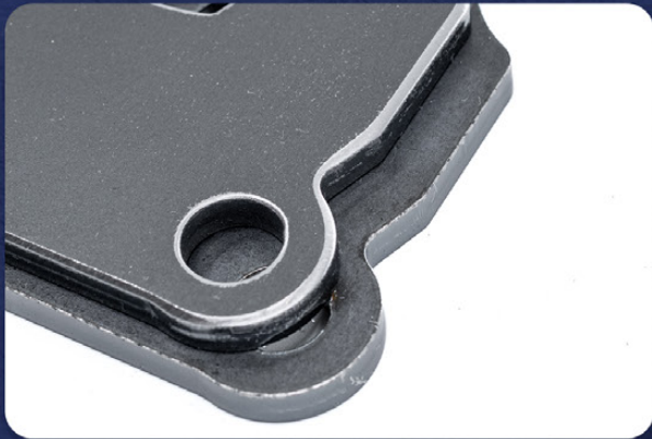
Deburring and edge rounding – steel
